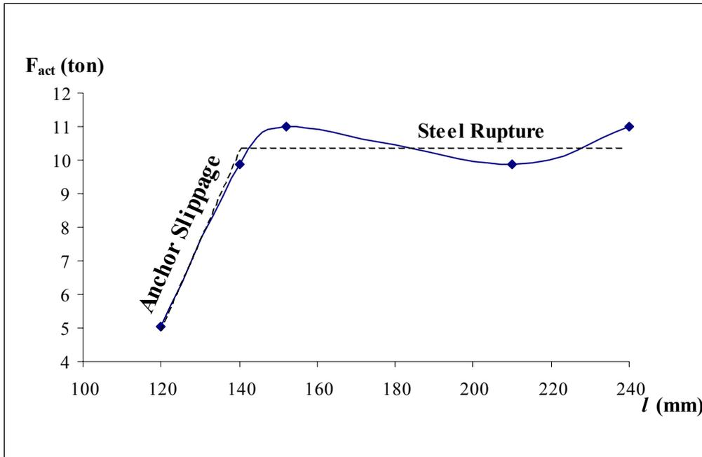
Fig. (10): Failure Force for Bonded  $\phi$  16 at Angle of  $\theta = 90^\circ$  Versus Embedment Length
