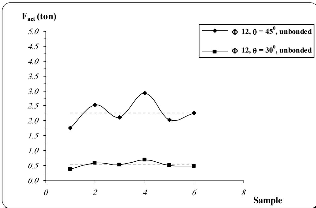
Fig. (11): Comparison for Different Embedment Angle for  $\phi$  12
