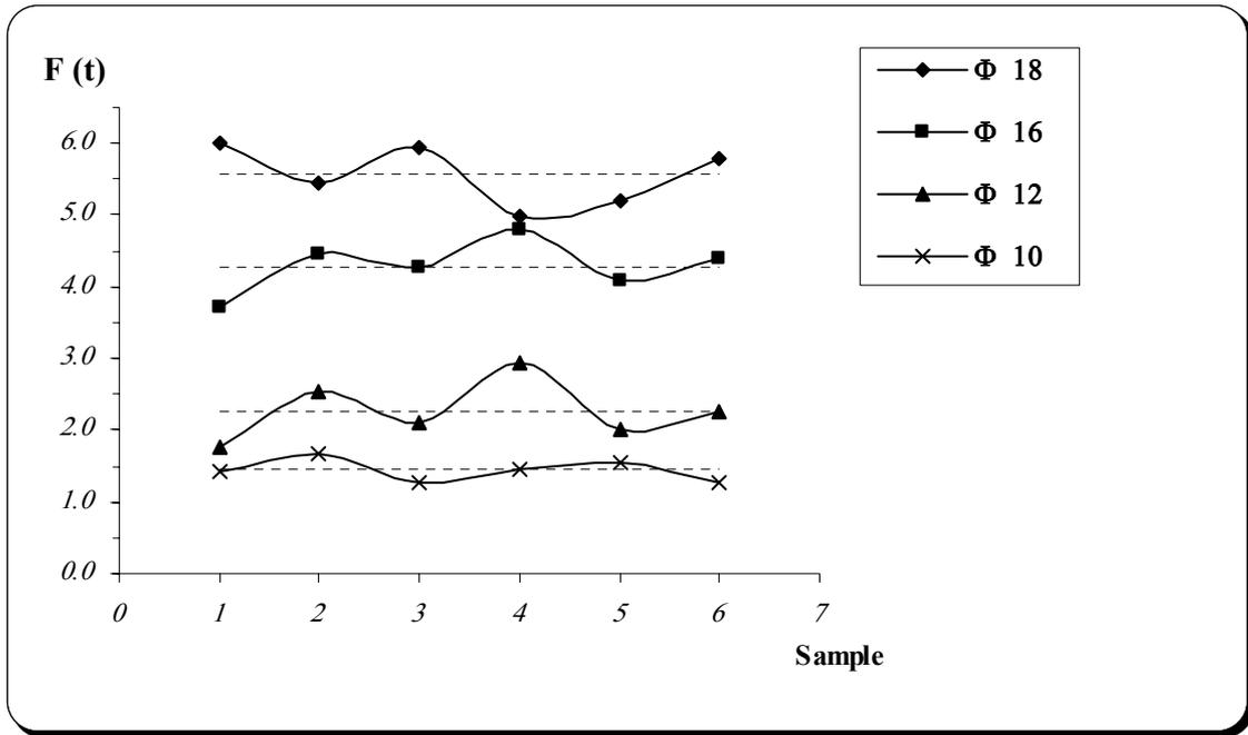
**Fig . (4): Results of Ubonded Anchor at Angles of  $\theta = 45^{\circ}$**
