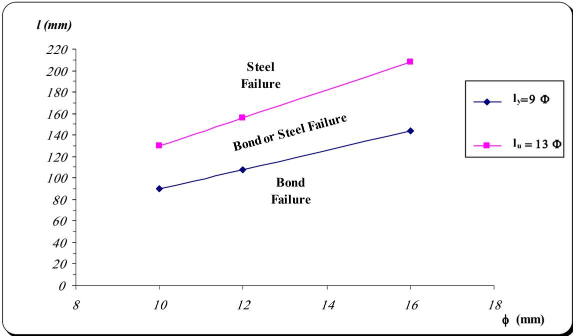
Fig. (8): Bounding Limits for Different Failure Modes,  $\theta = 90^\circ$
