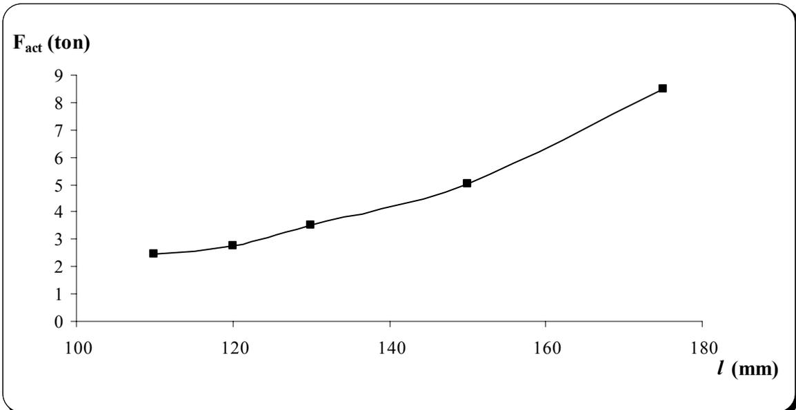
Fig. (9): Failure Force for Bonded  $\phi 16$  at Angle of  $\theta = 45^\circ$  Versus Embedment Length
