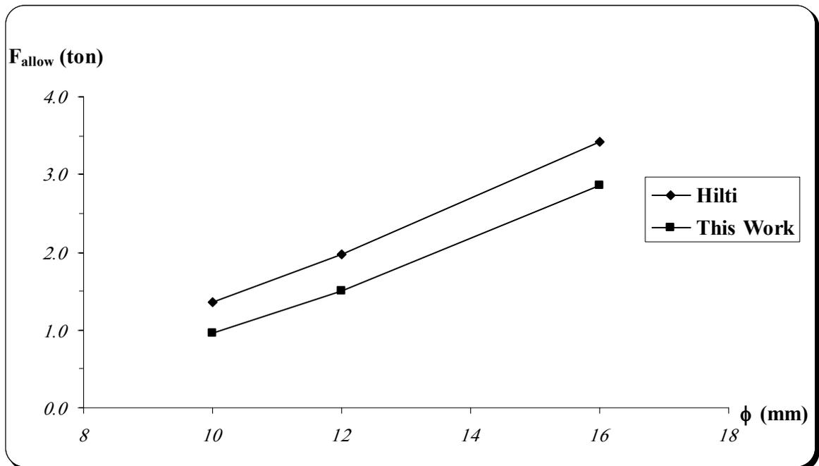
Fig. (13): Comparison of Unbonded Anchor at Angle  $\theta = 45^\circ$  with Hilti Values
