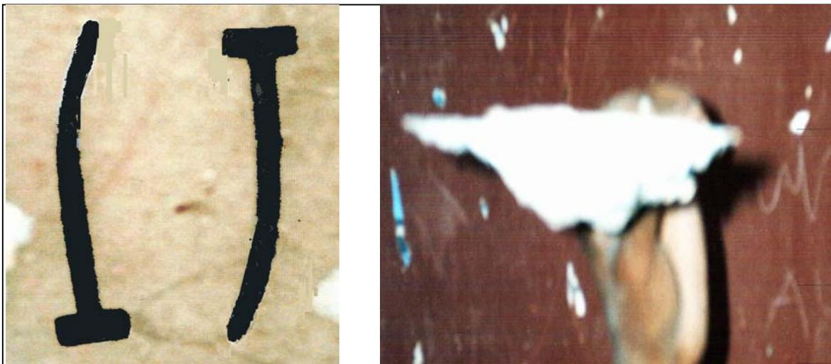
**Fig. (3): Base Material Mode of Failure**
