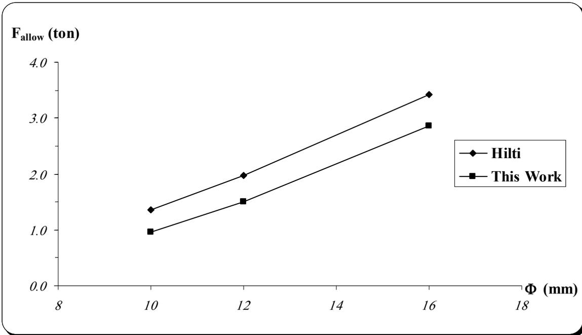
**Fig. (14): Comparison of Bonded Anchor at Angle  $\theta = 90^\circ$  with Hilti Values**
