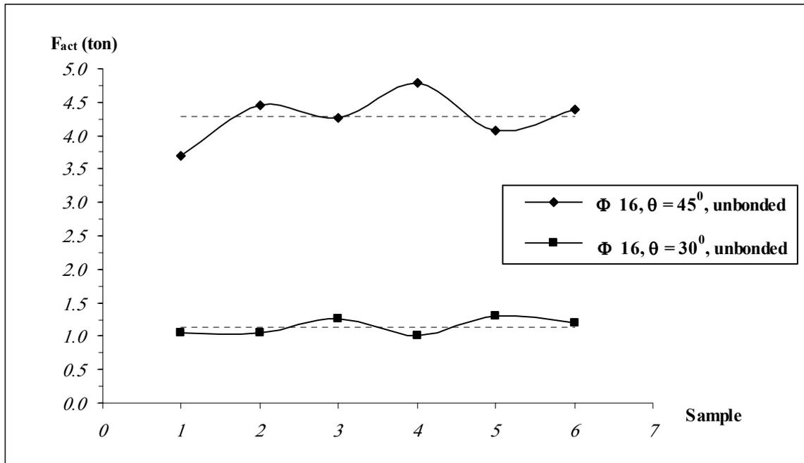
Fig. (12): Comparison for Different Embedment Angle for  $\phi 16$
