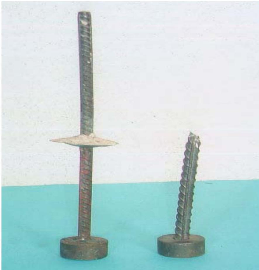
**Fig . (7): Slippage of Bars and Steel Rupture Failure Patterns**
