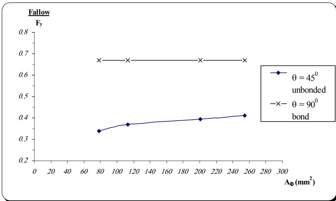
**Fig . (5): Relationship between Anchor Cross-sectional Areas and Allowable Force Ratios**
