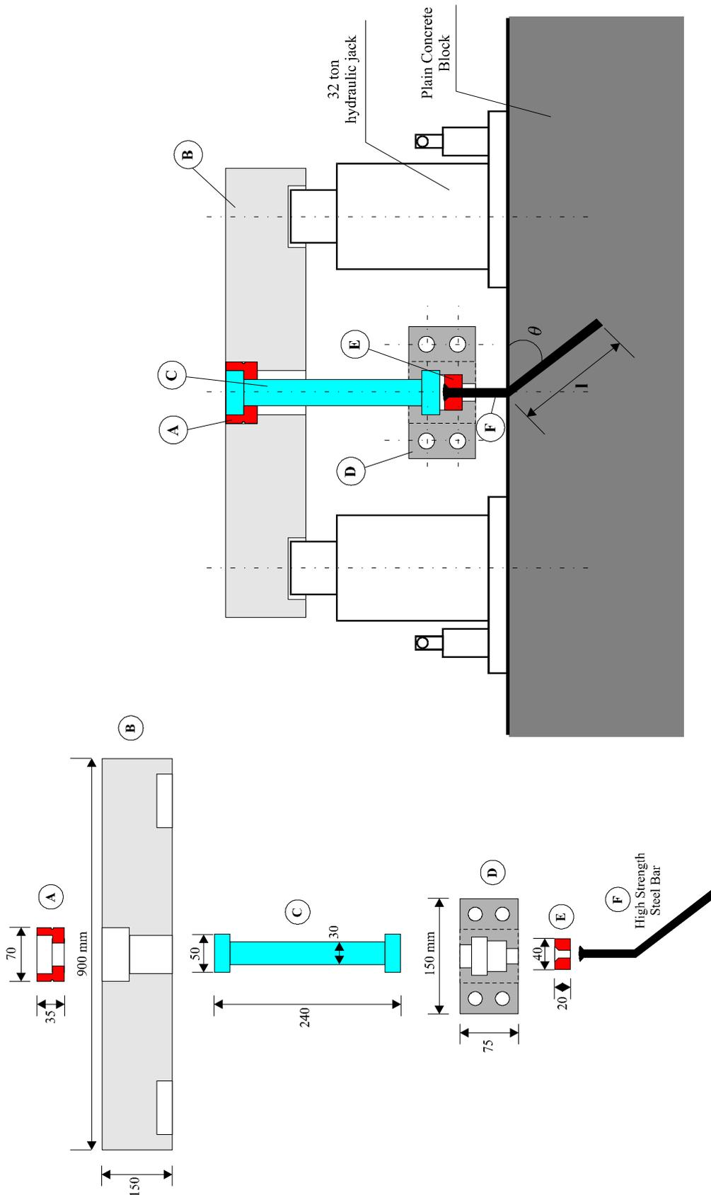
**Fig. (1): Schematic Layout for the Testing Pull-out Device**
